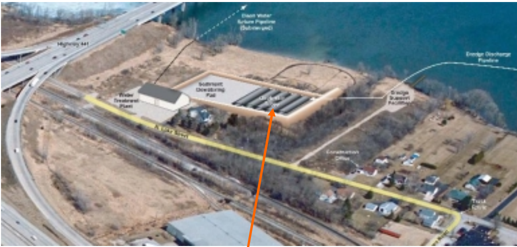
The layout of a dredging operation at Fox River. Geotube® containers are positioned in the center.
