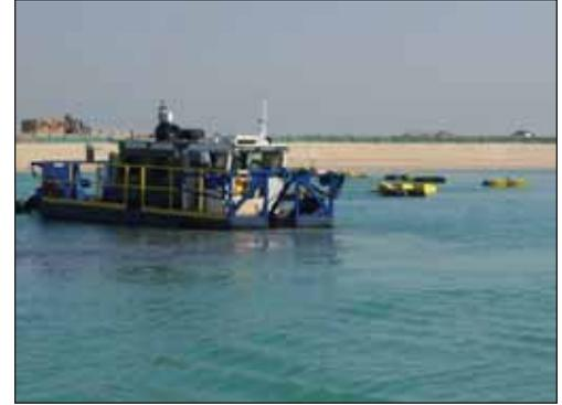
A Model 5012 LP removes silt from channels at a resort in the Middle East.
